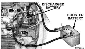
2. Connect one end of the other jumper cable to negative (-) post of booster battery. Connect the other end of the jumper cable to a good ground on the engine block of the vehicle with the discharged battery. Make sure a good connection is made, free of dirt and grease.
